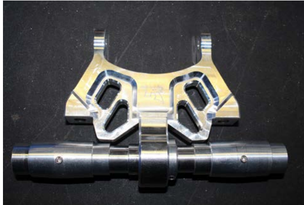
Fig. 2 - The eyelet on the pivot has Loctite applied and the bolt has been torqued to 40 Ft Lbs here prior to shipping.
