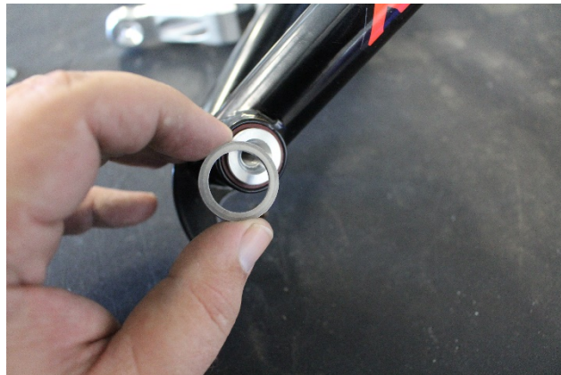
Fig. 3 – spacer shim location
