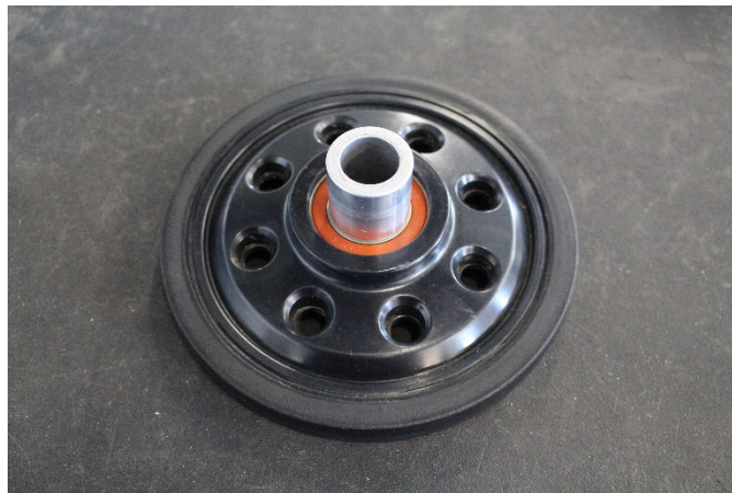
Fig. 5 – rear carrier wheel with kits spacers
