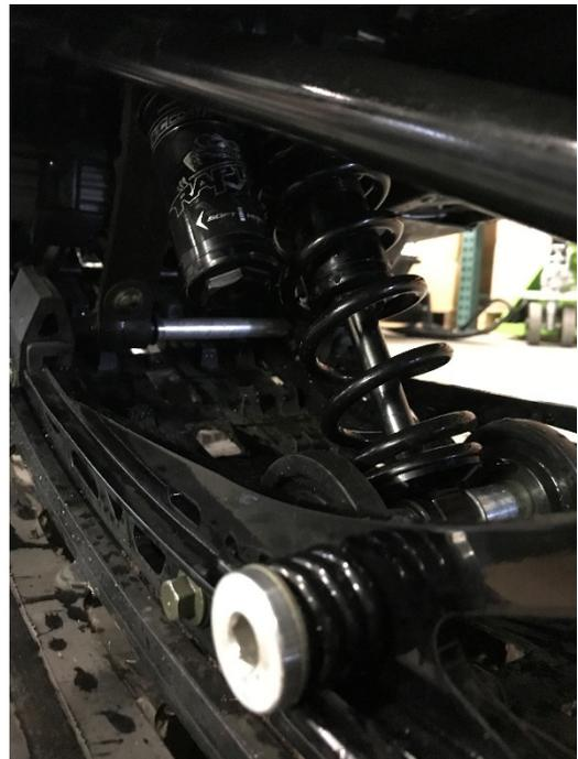
*Figure 1. Front Track Shock Mounting Position*
