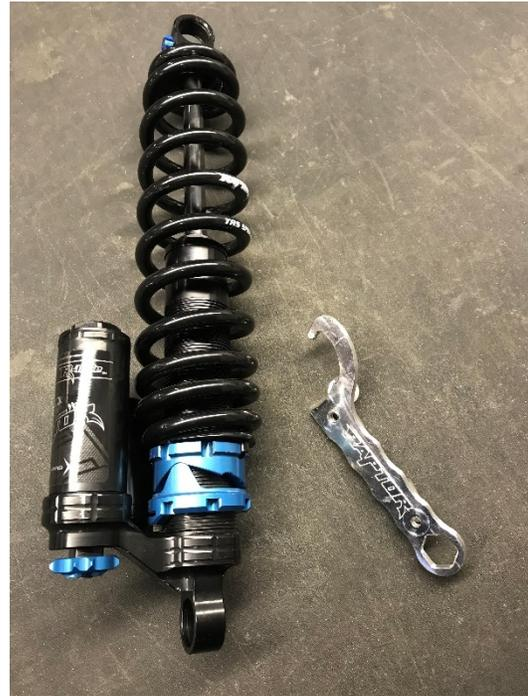
*Figure 2. Rear Track Shock with Quick Cam Adjuster*
